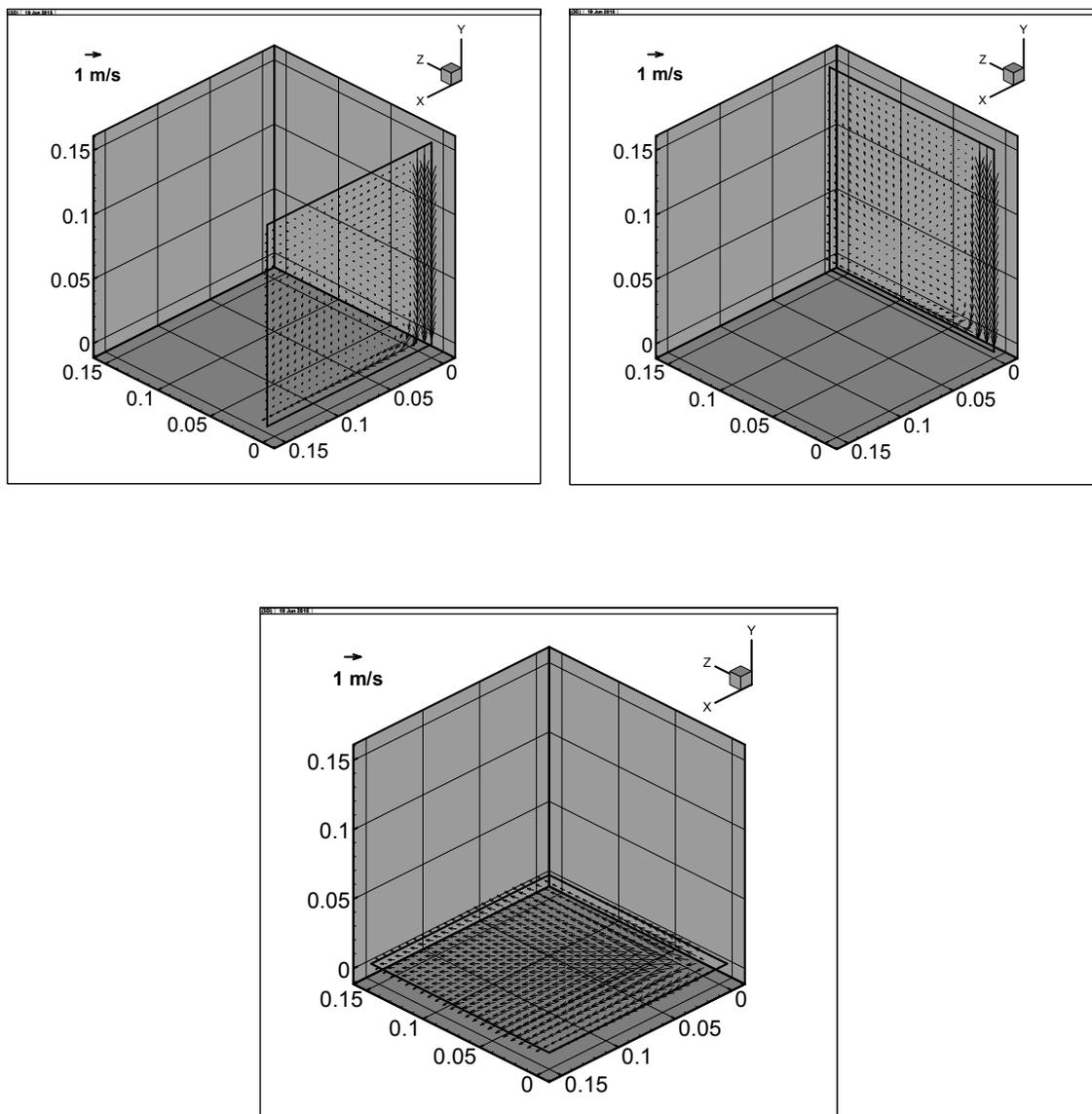
**Fig. 4** Vector field in three planes for selective planes for  $Re = 1000$  and  $q = 1000 \text{ W/m}^2$
