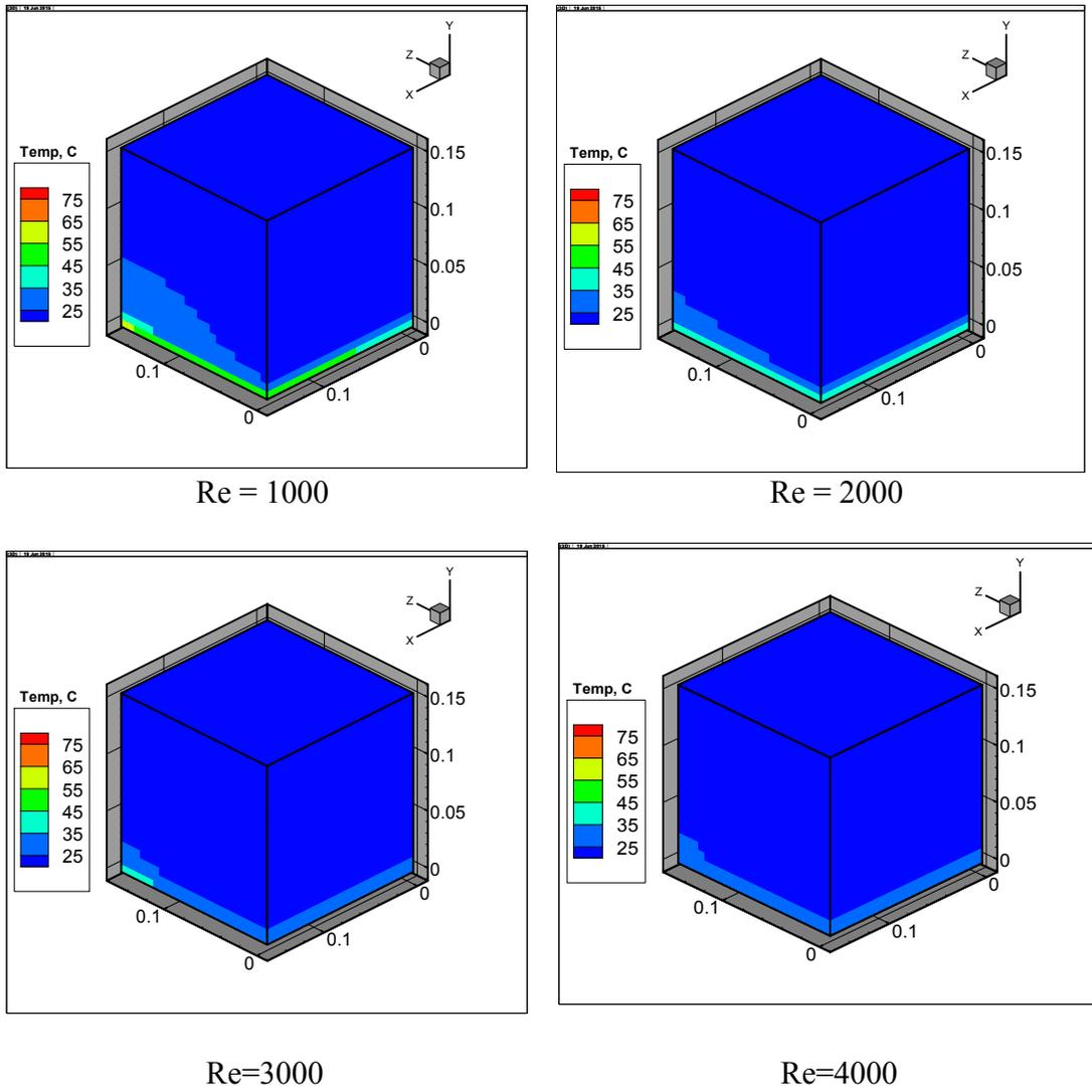
**Fig.2** Isotherms for jet domain for different Reynolds number with  $q = 1000 \text{ W/m}^2$
