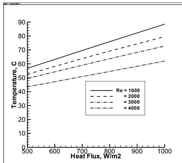
**Fig. 6** Plate temperature variations with heat flux for different Reynolds number.
