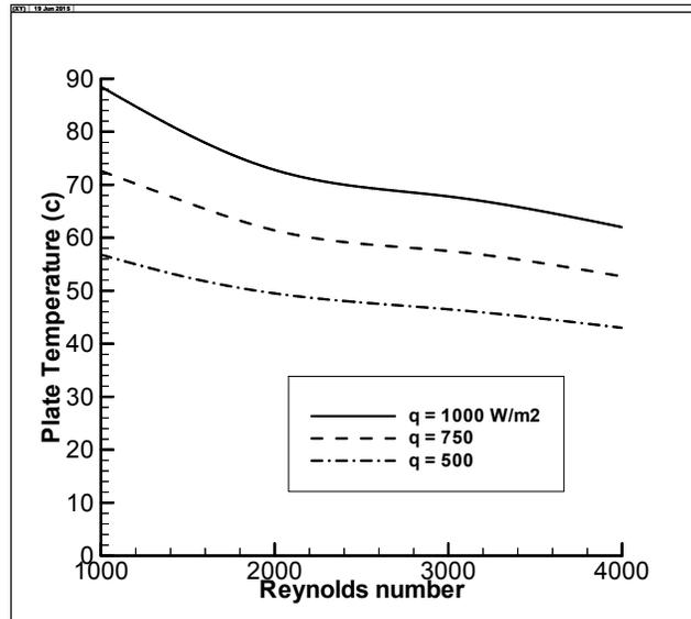
**Fig. 5** Plate temperature variations with Reynolds numbers for different heat flux.
