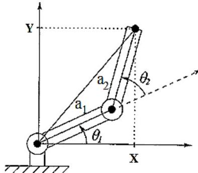
Figure 1: Two-link robotic arm <sup>[10]</sup>.
