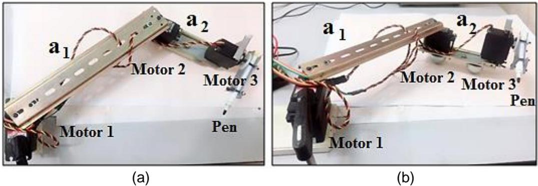
**Figure 2: Practical two-link robotic arm design in two sides: (a): top view (b): side view.**
