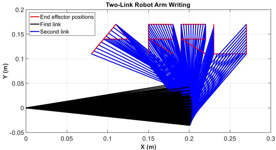
**Figure 7: Simulation of two-link robotic arm motion using designed NN.**
