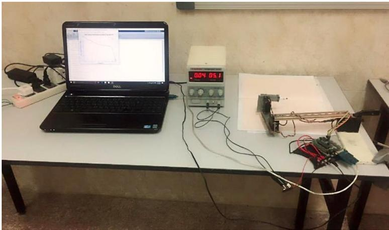
**Figure 6: Experimental work of the two-link robotic arm with three servomotors and SSC-32 Servo controller at ARRU-CSED-UOT.**
