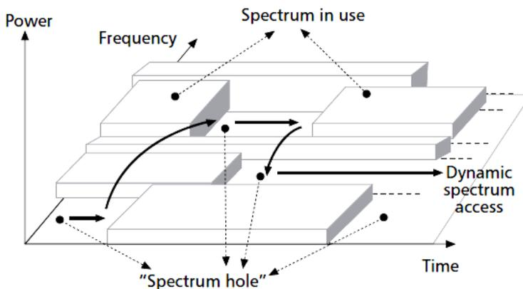
Figure 1. Spectrum-hole concept.
