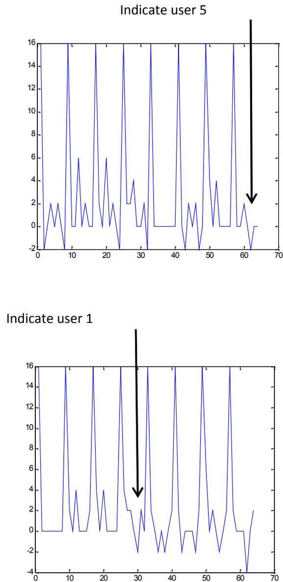
**Figure(3).** Output of equations (3,4) for complementary and not compatible complementary of Golay code sequences
