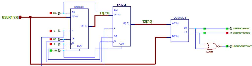
Figure(4-b) implementation of user received signal tracker
