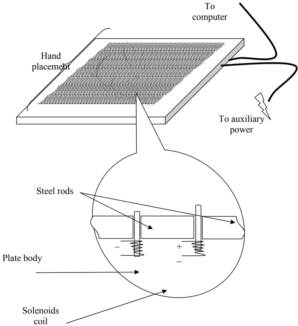
The workspace is about 20 cm by 30 cm i.e 600 cm square. The effective mass in each direction is 95 grams while the maximum force output is about 6 Newtons. The workspace of the current is limited by the solenoids. Future designs will utilize rotary motors and capstan drives, realizing large workspaces yet maintaining a low profile package.
