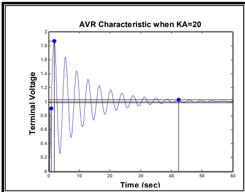
Figure 2 Terminal voltage of the generator with KA = 1 and KA = 20
