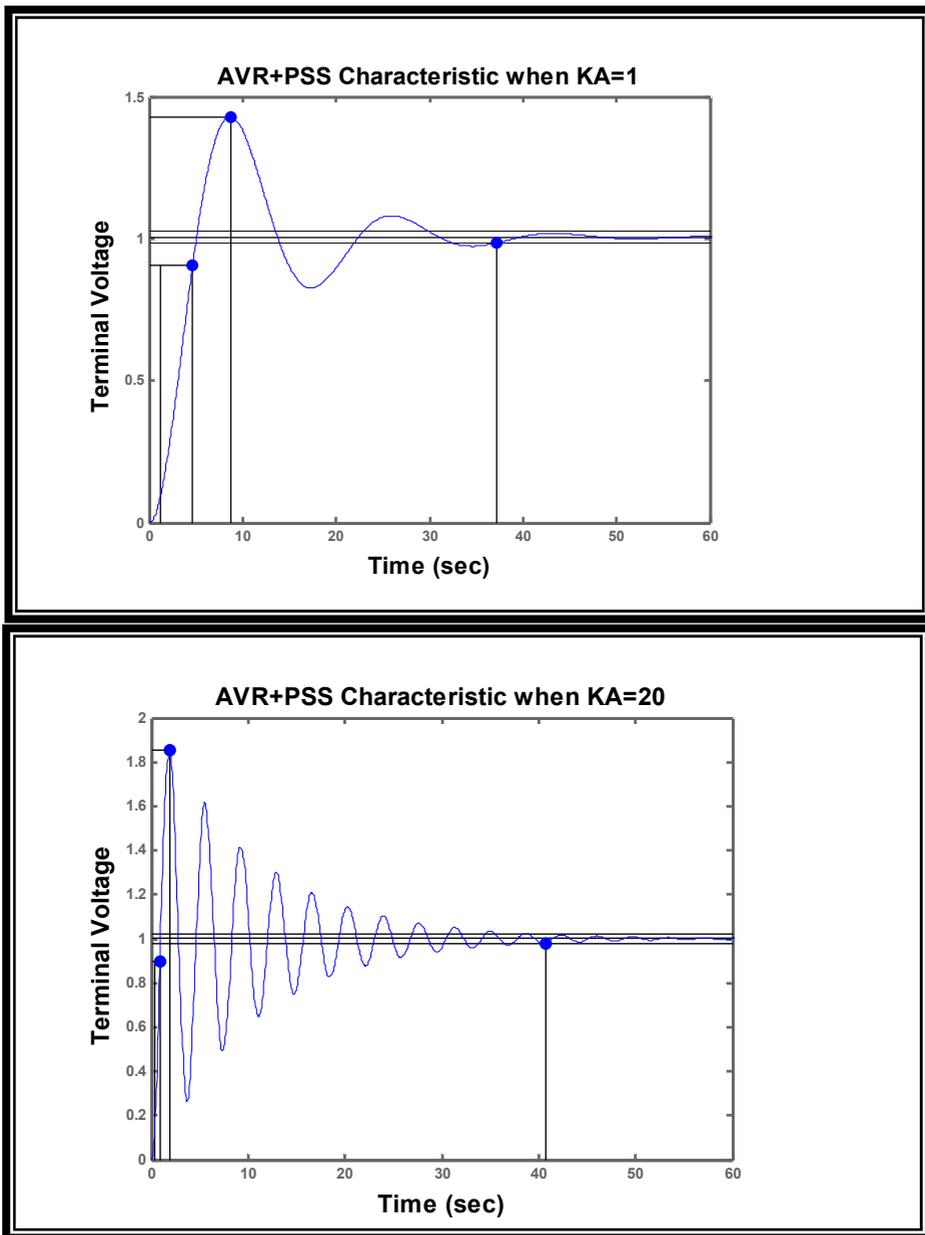
Figure 6 Terminal voltage of the generator with KA = 1 and KA = 20
