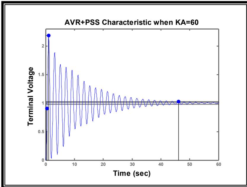
Figure 7 Terminal voltage of the generator with  $K_A = 40$  and  $K_A = 60$
