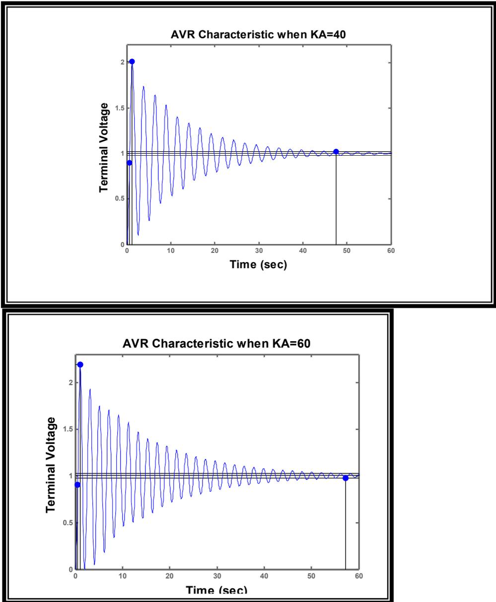
Figure 3 Terminal voltage of the generator with KA = 40 and KA =
