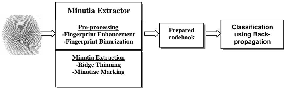
Figure 2 Fingerprint Recognition System
