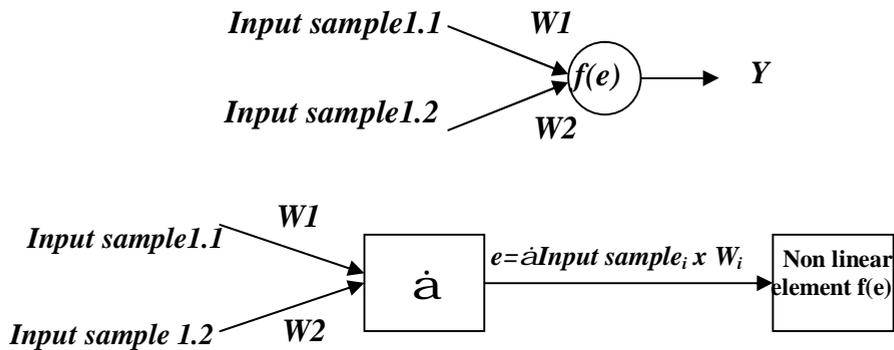
Figure 6 Backpropagation neuron unit
