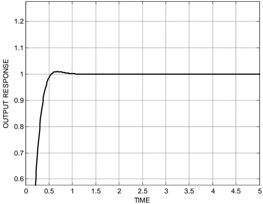
**Fig. (7) The response of PID controller using genetic al first run.**
