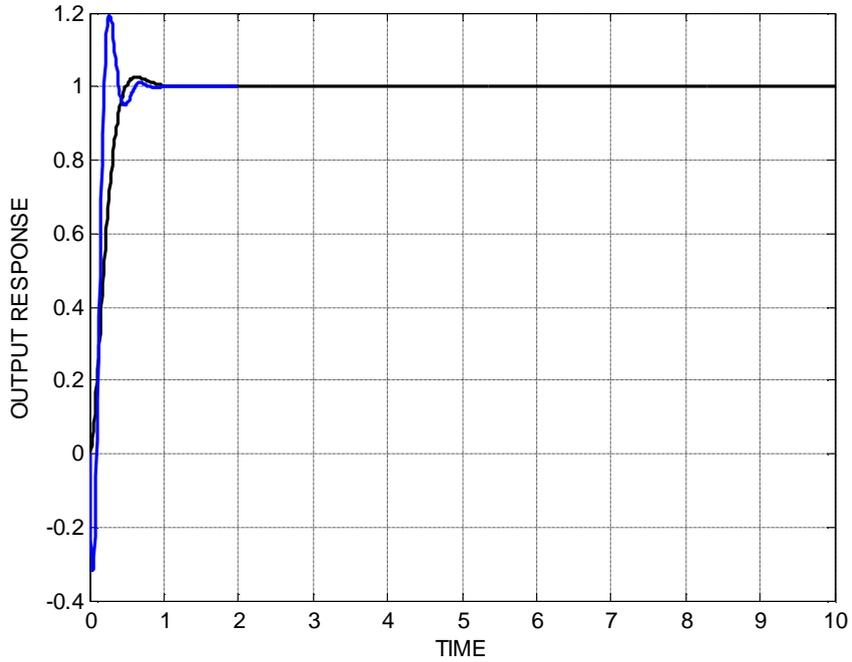
**Fig. (13 ) The responses of PID controller using genetic algorithm and ITAE(blue line for ITAE and black for GA).**
