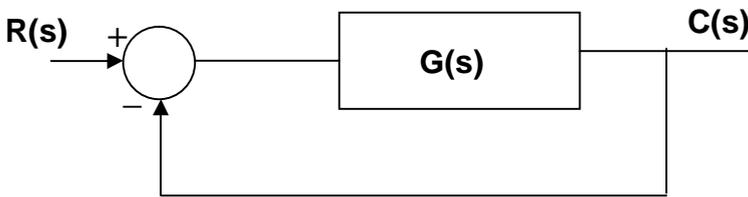
Fig. (5) Closed loop system
