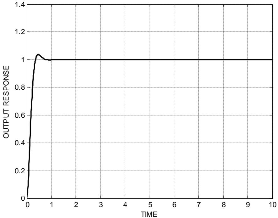
**Fig. ( 9) The response of PID controller using genetic algorithm for third run.**
