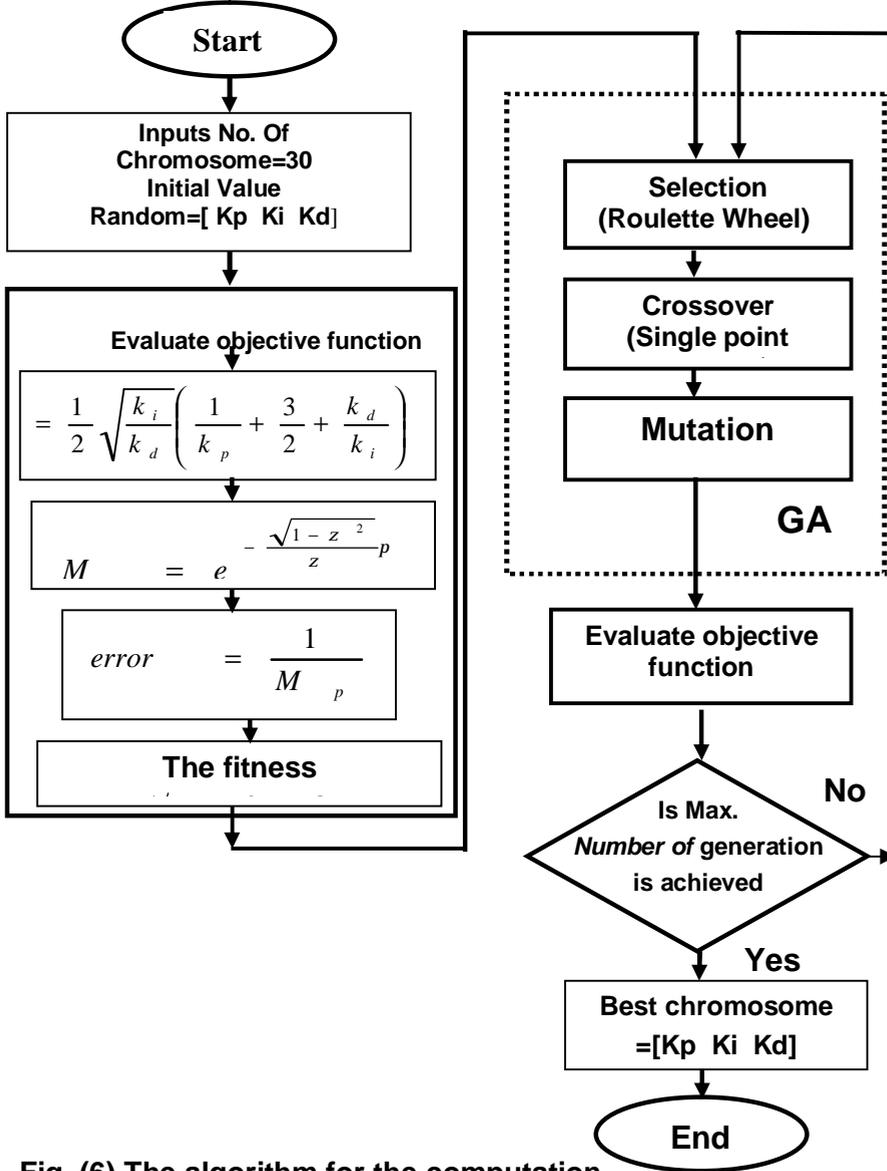
Fig. (6) The algorithm for the computation of PID parameters using genetic algorithm.
