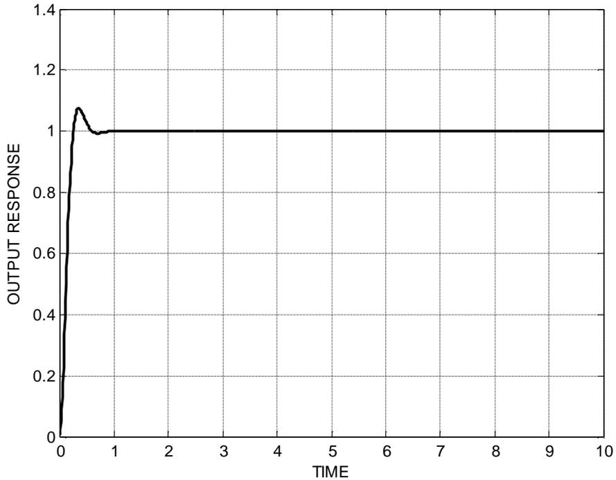
**Fig. (8 ) The response of PID controller using genetic algorithm for second run.**
