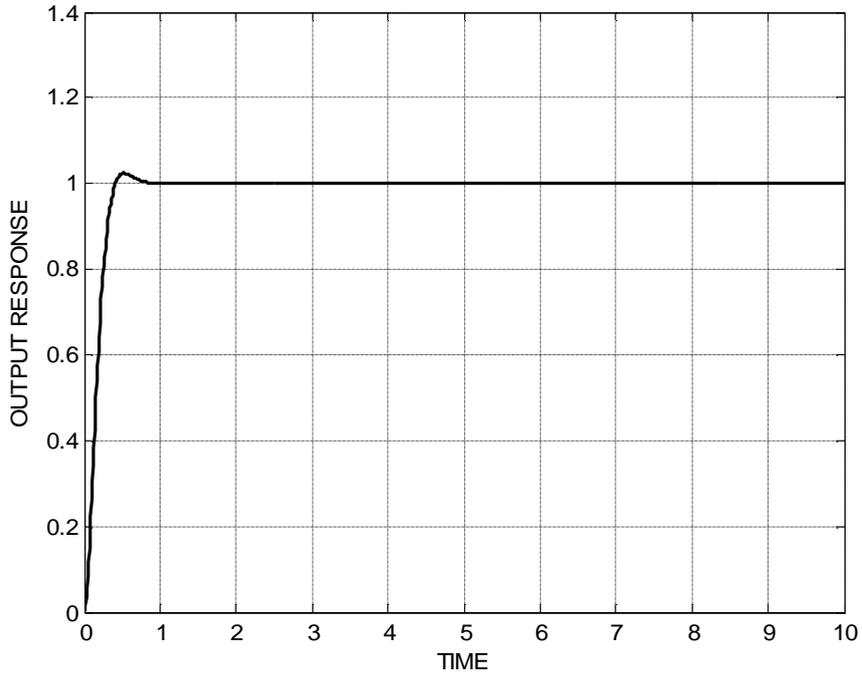
**Fig. (11 ) The response of PID controller using genetic algorithm for fifth run.**
