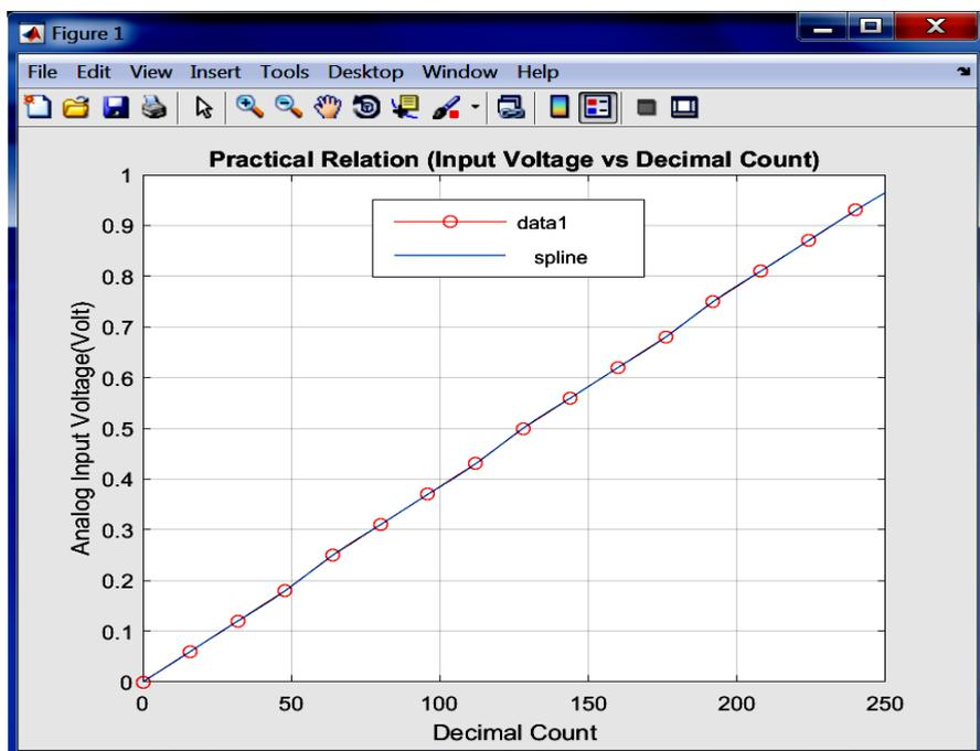
**Figure 5. Practical Results of the Proposed A/D Converter Circuit with 16 measurement points.**
