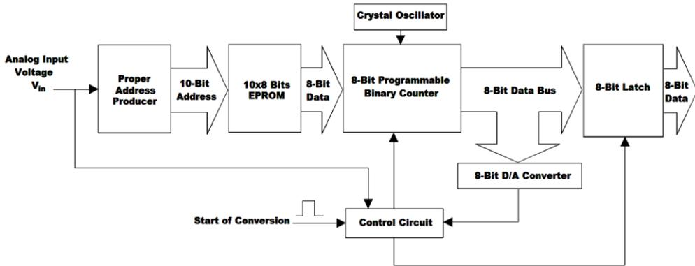
Figure 2. Block Diagram of the Proposed Circuit.
