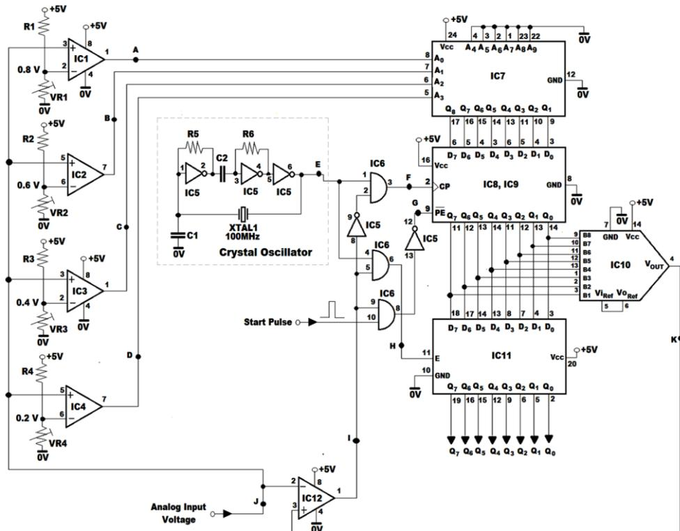
Figure 3. Circuit Diagram of the Proposed A/D Converter Circuit.
