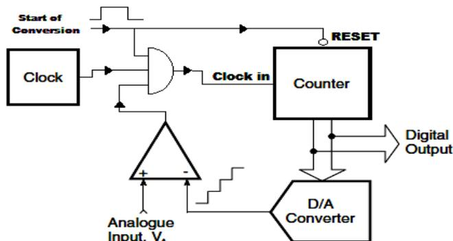
Figure 1. The Circuit Diagram of the Counter-Ramp A/D Converter.
