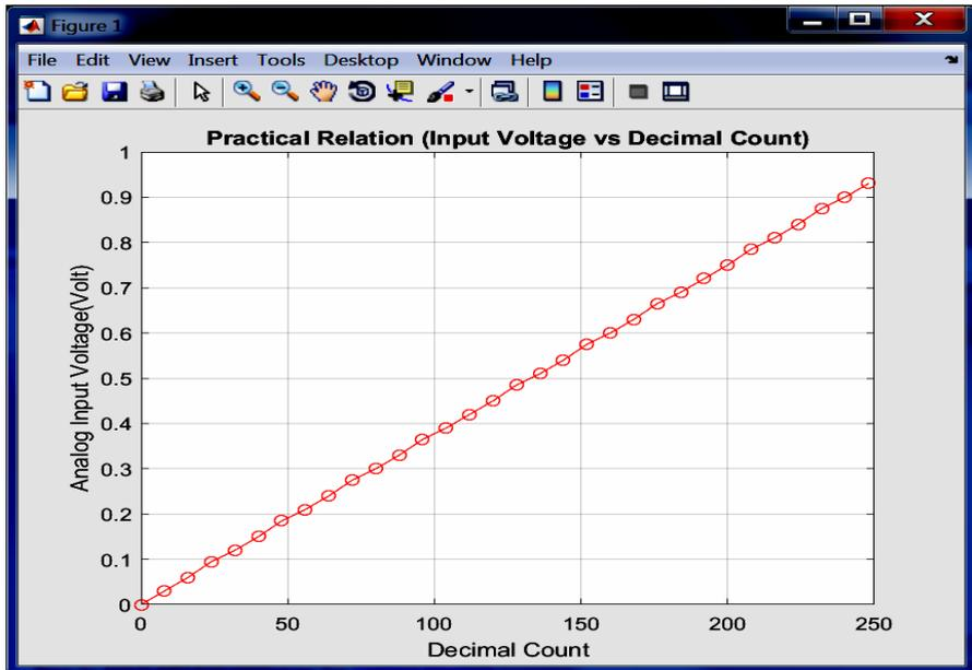
**Figure 6. The relation between the analog input voltage and decimal representation of digital output data with 32 measurement points.**
