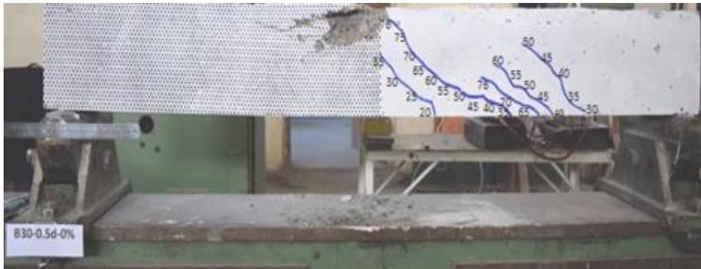
Figure 17: Crack pattern of beam (B30-0.5d-0)
