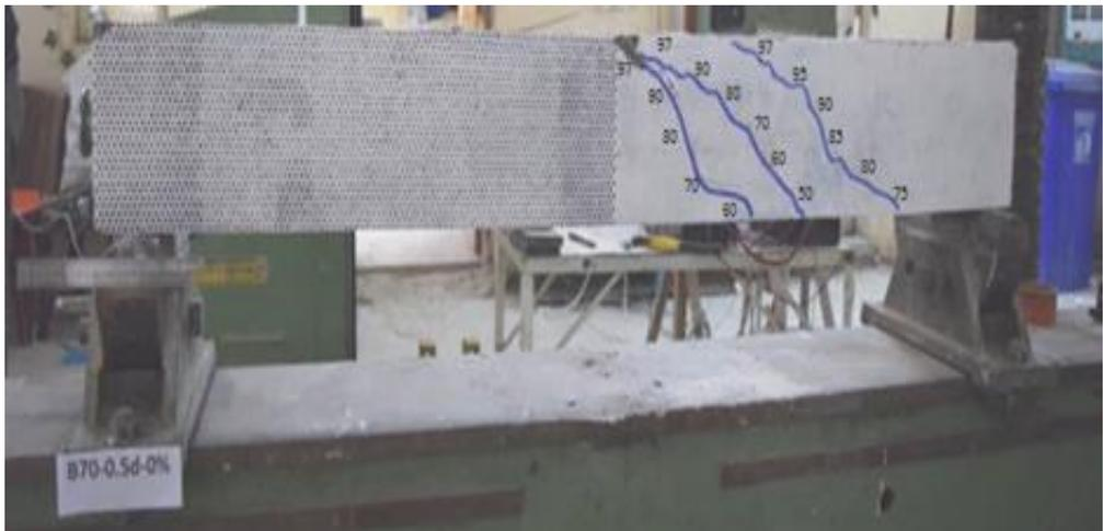
**Figure 29: Crack pattern of beam (B70-0.5d-0)**
