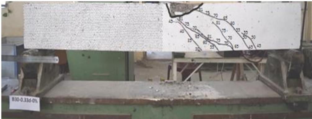
**Figure 20: Crack pattern of beam (B30-0.33d-0)**
