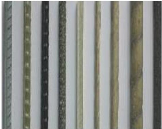
**Figure 3: A different type of FRP rebar**
