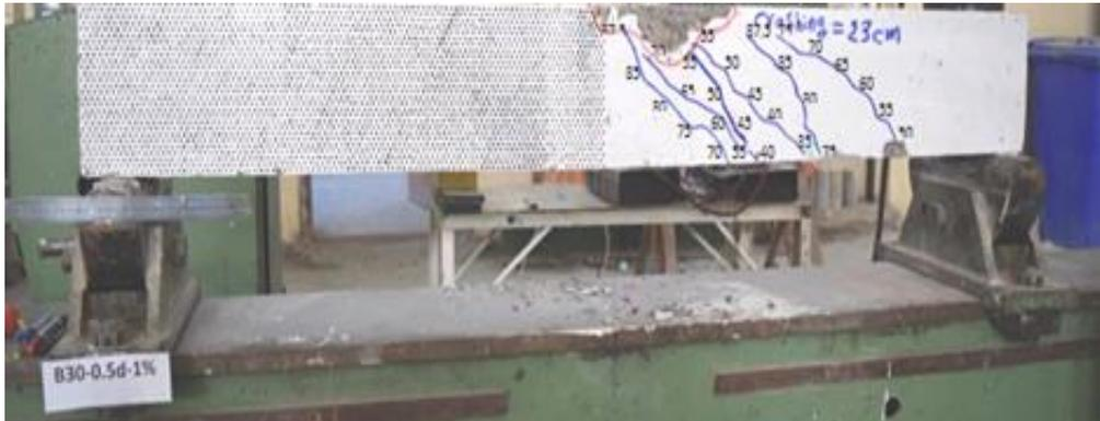
**Figure 19: Crack pattern of beam (B30-0.5d-1)**
