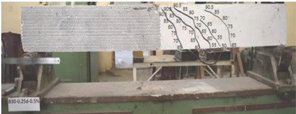
**Figure 24: Crack pattern of beam (B30-0.25d-0.5)**
