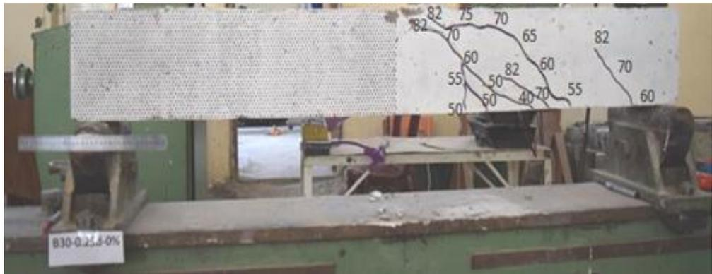
**Figure 23: Crack pattern of beam (B30-0.25d-0)**
