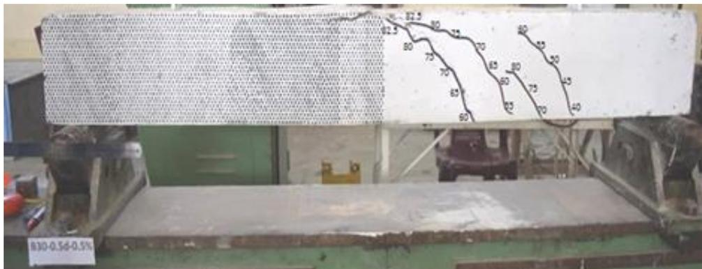
Figure 18: Crack pattern of beam (B30-0.5d-0.5)
