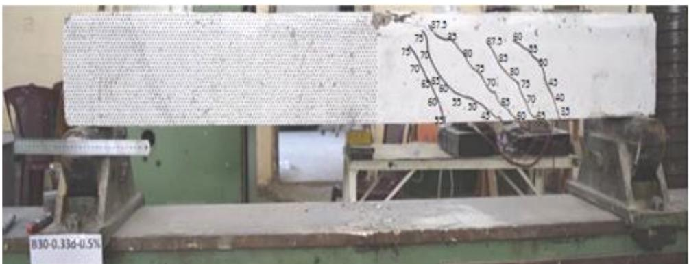
**Figure 21: Crack pattern of beam (B30-0.33d-0.5)**
