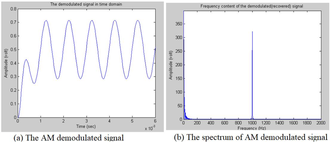
Figure (9): AM mode demodulated signal.
