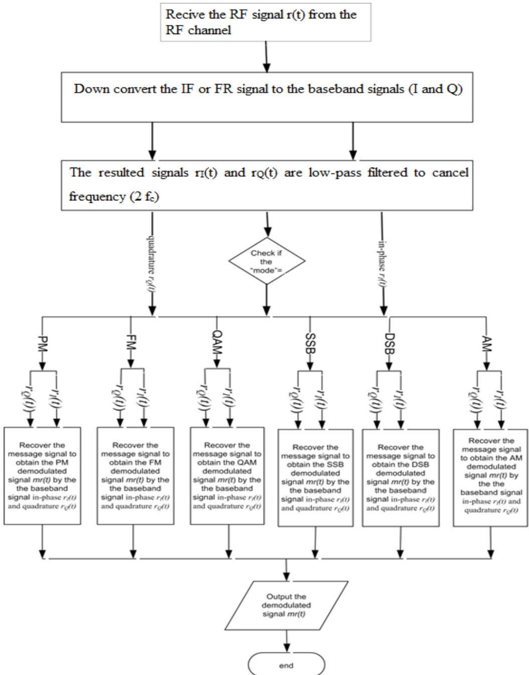
Figure (5): The general flowchart of the implemented demodulator.
