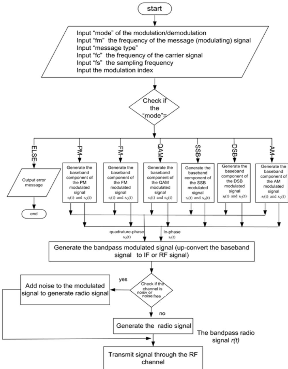
Figure (4): The general flowchart of the implemented modulator.
