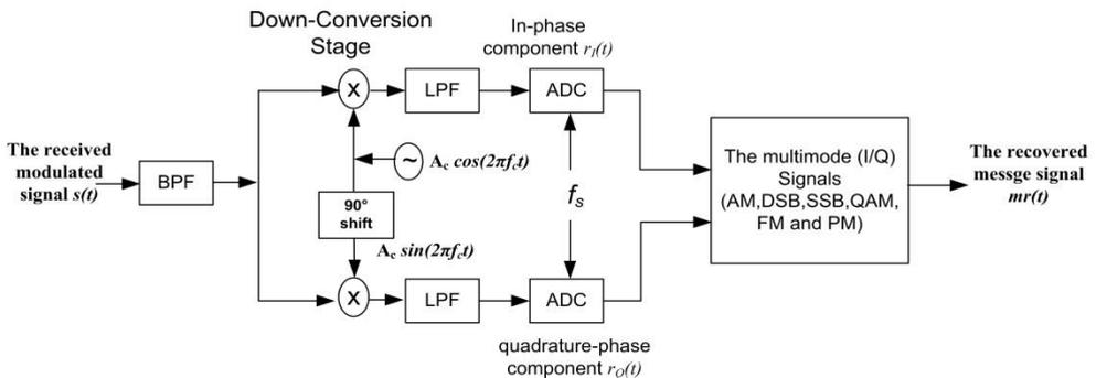
Figure (2): General block diagram of the demodulator section.
