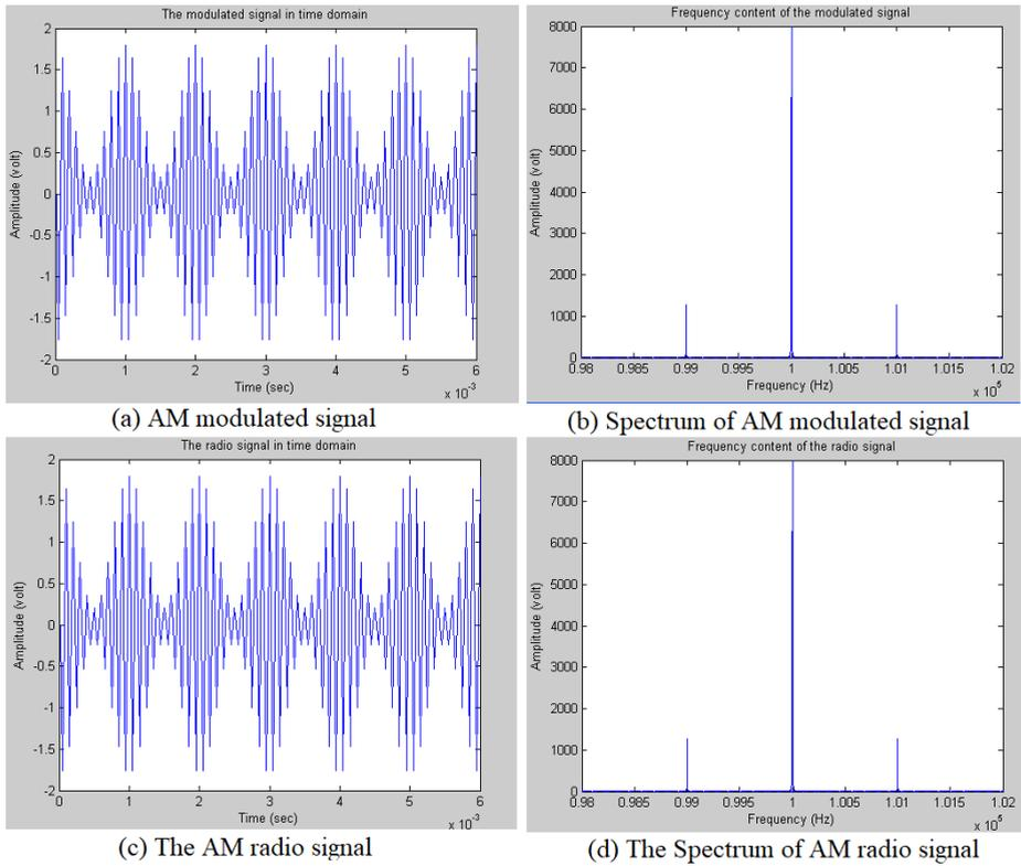
Figure (8): AM mode modulated signal.
