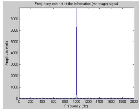
(b) Spectrum of Modulating signal
