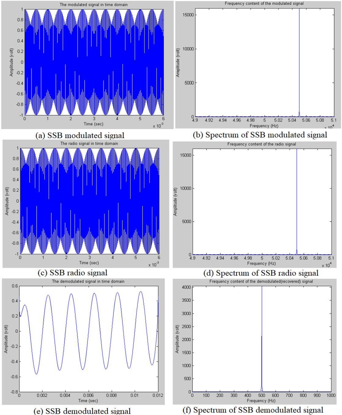
Figure (11): SSB modulation and demodulation results.
