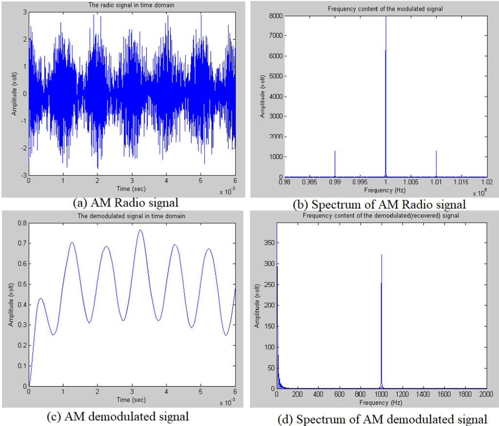
**Figure (10): AM radio and demodulated signals using noisy channel.**
