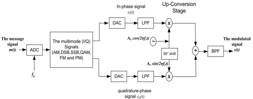
Figure (1): General block diagram of the modulator section
