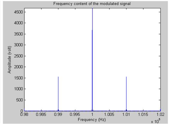
(b) Spectrum of PM modulated signal
