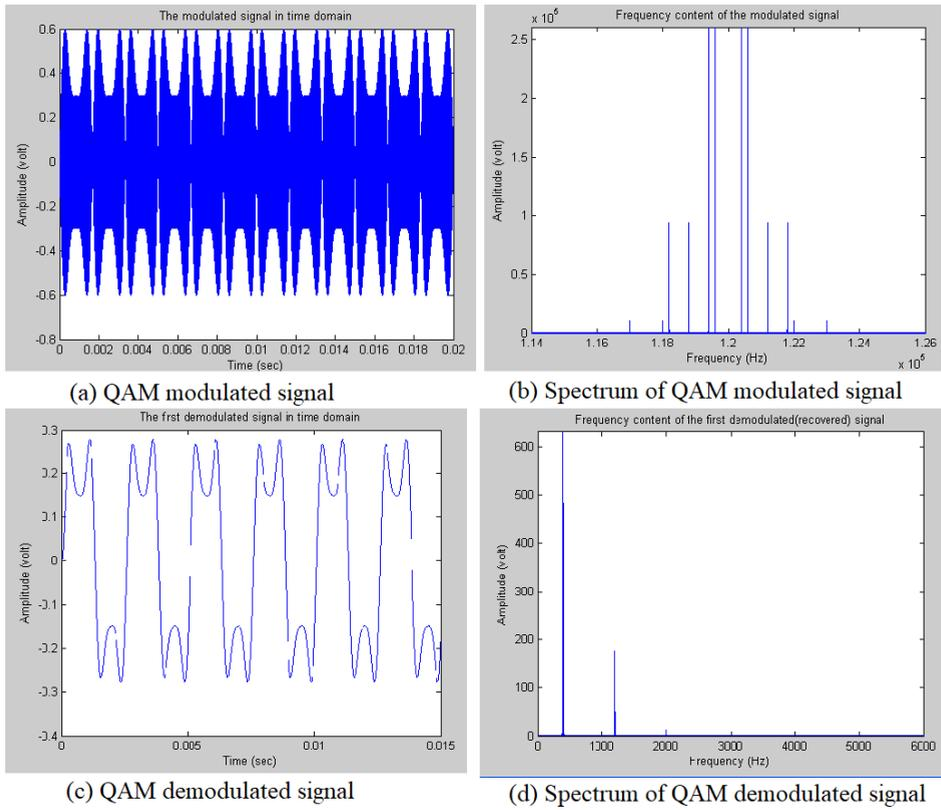
Figure (14): QAM modulation and demodulation results.
