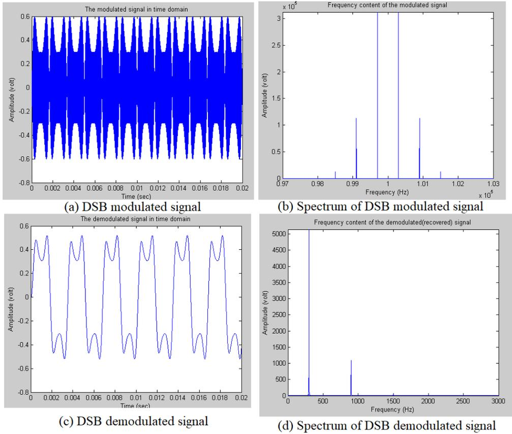
**Figure (13): DSB modulation and demodulation results.**
