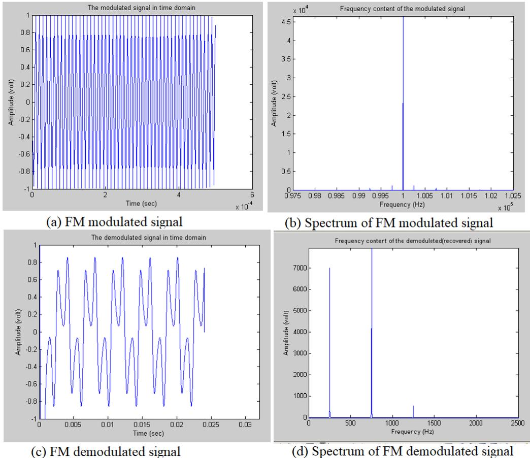
**Figure (15): FM modulation and demodulation results.**
