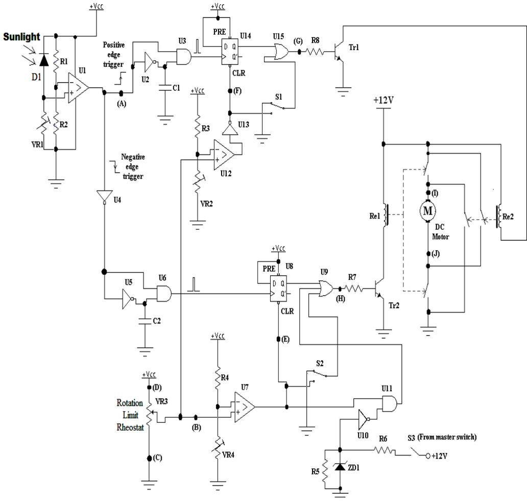
Figure (4): The complete circuit diagram of the proposed system.
