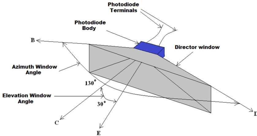
**Figure (2): The photodiode and its light director of the proposed system**
