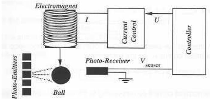
**Figure (1): Simplified Magnetic levitation System Diagram**
