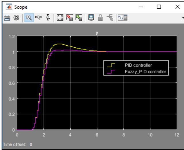
Figure (6): Comparisons of PID and Fuzzy PID control.
