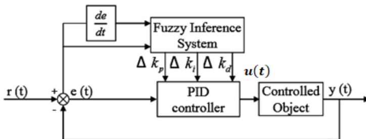
**Figure (2): Basic structure for “Self-Tuning parameter Fuzzy PID Controller”**
