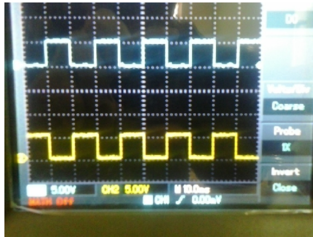
Figure 16: Microcontroller Generated Square Waves Displayed on the Oscilloscope (Scale : 5 V/div, 10 ms/div).
