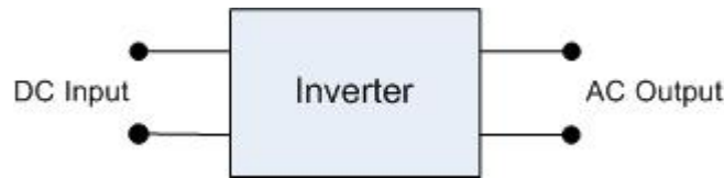
Figure 1: Block Diagram of an Inverter.
