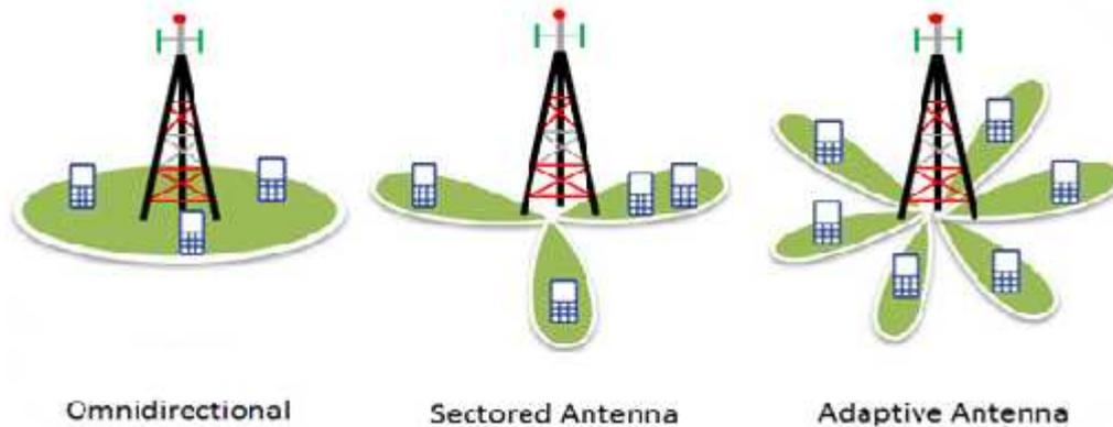
Figure (1) - Base Station Antenna Configuration
