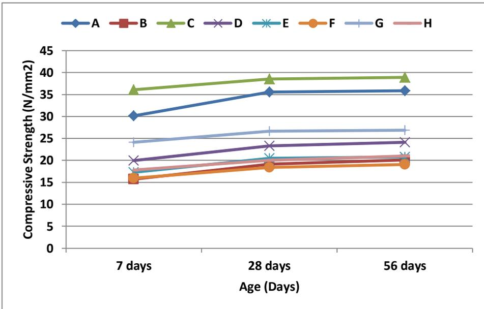
Figure 4. compressive strength of all types of mortars under accelerated curing
