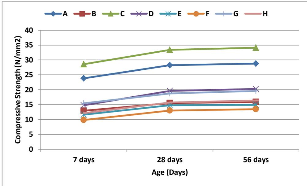
Figure 3. compressive strength of all types of mortars under normal curing
