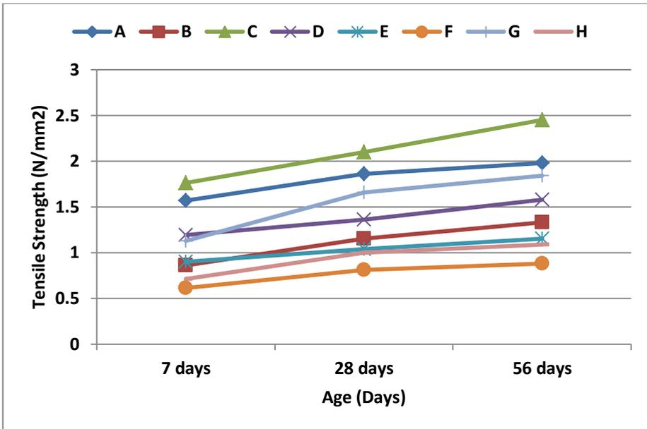
Figure 6. Tensile strength of all types of mortars under accelerated curing
