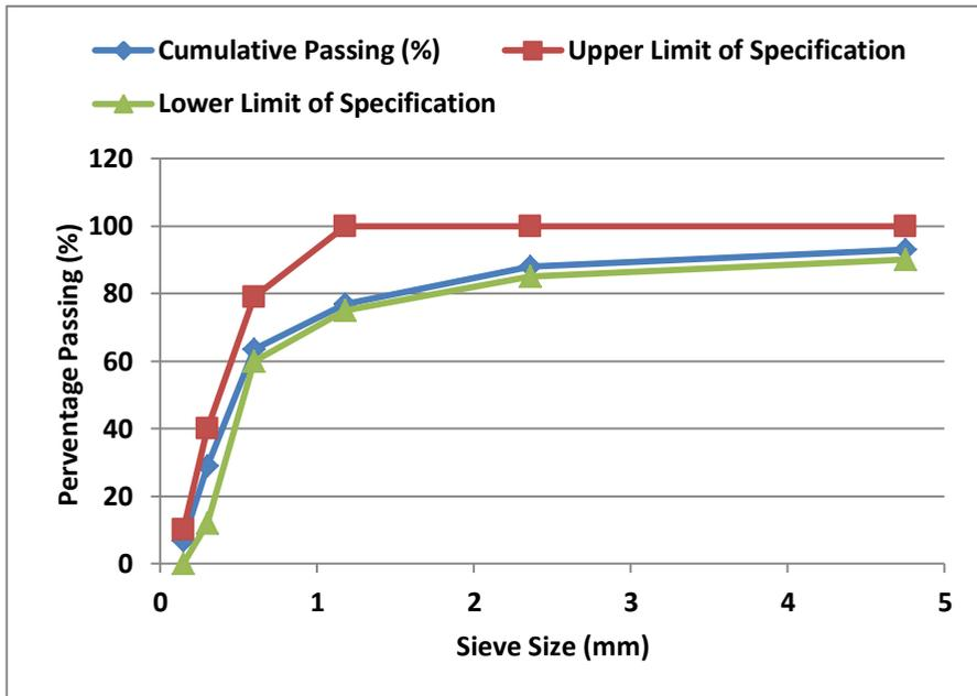
Figure 1. Grading curve for natural sand with grading limits in zone 3.
