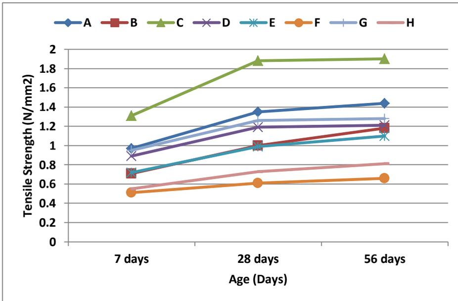
Figure 5. Tensile strength of all types of mortars under normal curing
