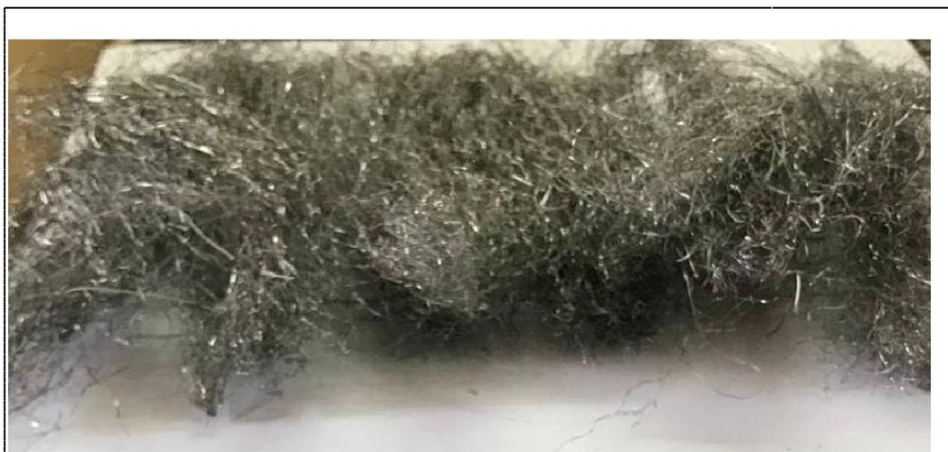
**Figure 1. The micro steel fibers used in the present study**
