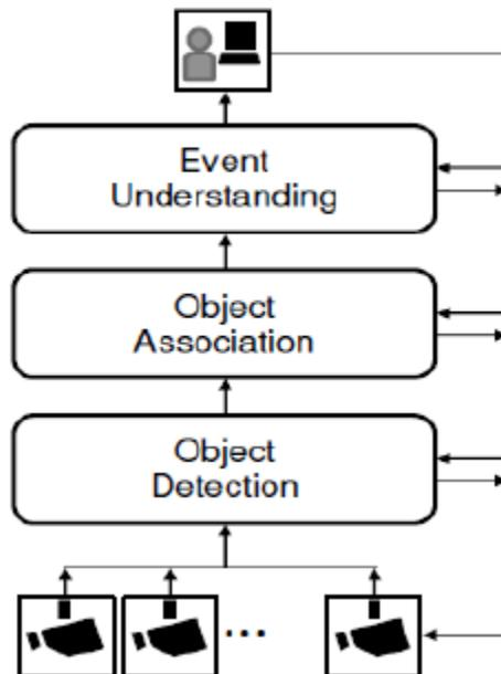
Figure (1) A diagram of A General Video-Based Surveillance System
